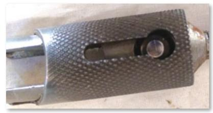
This is the risk: the pin and sleeve are almost correct but the sleeve is a little twisted and the pin is held in.
