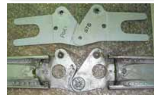
New steel root-fittings are installed, replacing the original aluminium fittings.
