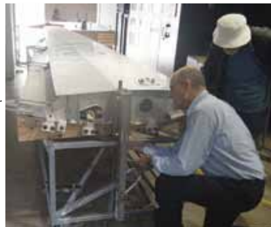
Ian Bent installing the expanding pin into the starboard wing of VH-XQO, in the CAMIT factory, whilst the starboard jig was being perfected, behind one of CAMIT's huge numerically-controlled machining centres. George Markey, head of ARMCOM, the holder of the licence to implement the modification, and the owner of the jigs, is looking on.
