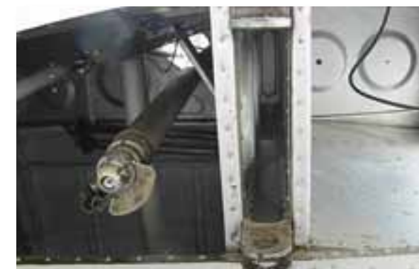
ABOVE: The side of the fuselage of VH-XQO removed to allow access for replacement of the lower wing carry-through member. Before the carry-through member can be removed, a jig must be attached to locate the new carry-through member with similar accuracy to that of the wing root fittings (obviously, they must fit one another or it will be impossible to rig the glider). The replacement carry-through member is of heavier section as well as being made of a superior material.
