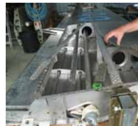
The starboard wing of VH-XQO, with the root fitting and the internal reinforcing strap (which runs from the root to rib#4) removed. Note the excellent condition of the interior of the wing.
