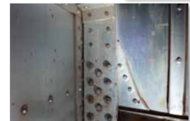
The Blaniks can regain airworthiness either through reinforcements to existing material, or with newly manufactured parts.
