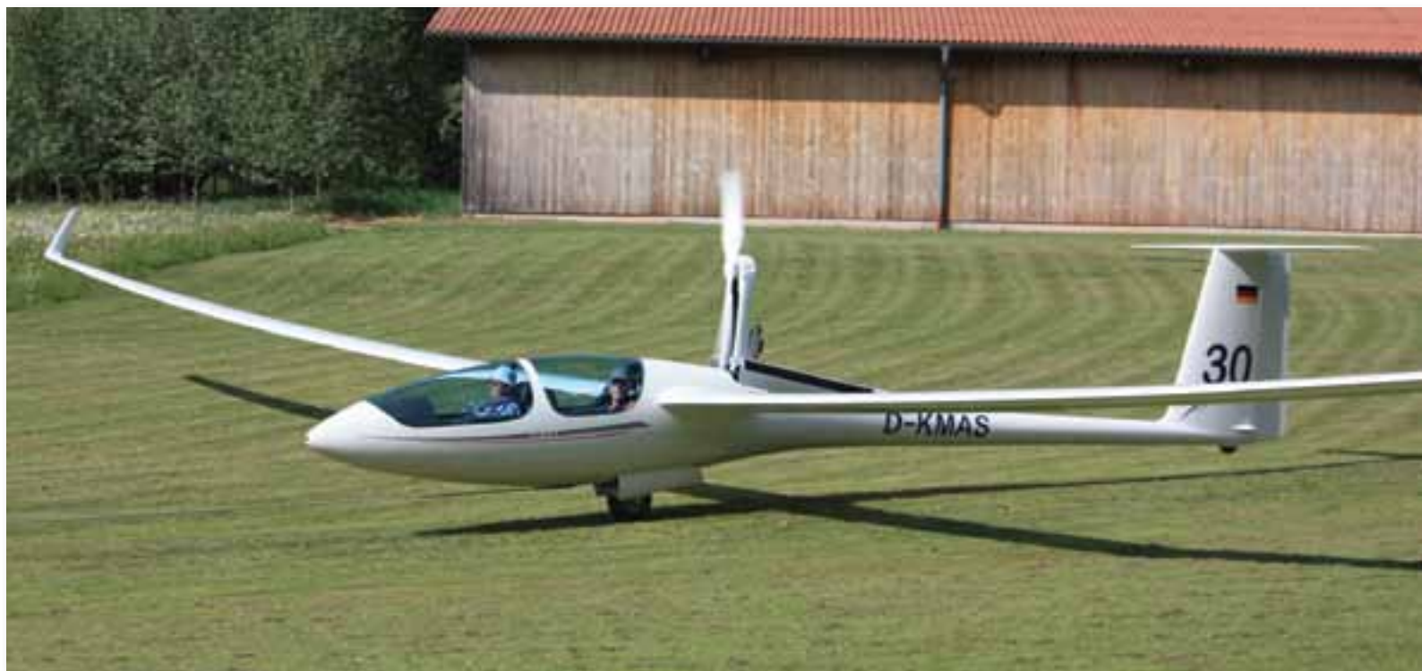
ABOVE: The two-piece canopy and elegant lines inherited from the ASH 25 give the ASH 30 Mi a typical 'Schleicher look', also evident when looking at the wing.
