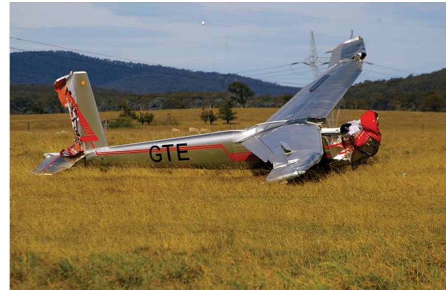
Southern Tablelands GC Blanik showing the collision damage to tail surfaces and ground impact damage elsewhere.
