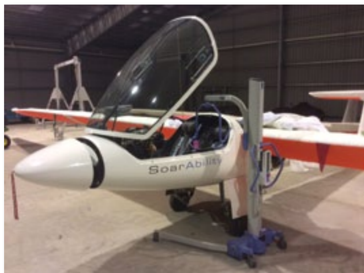
BOTTOM: The cockpit of the ASK21Mi. The rudder hand control lever is just below the blue handbrake lever.
