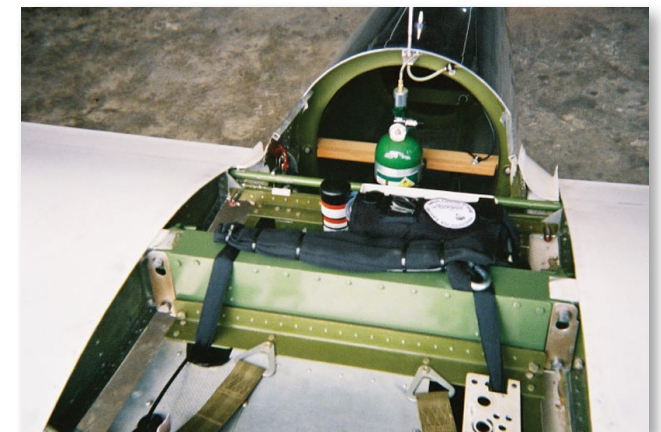
An installation of a Ballistic Recovery System (BRS) in a glider.
