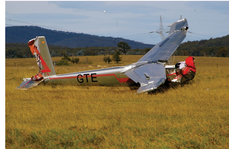
Southern Tablelands GC Blanik showing the the collision damage to tail surfaces and ground impact damage elsewhere.
