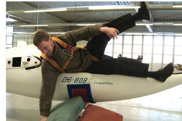
The NOAH System is an airbag that inflates and pushes the pilot to level of the cockpit, enabling a roll rather than a climb out.
