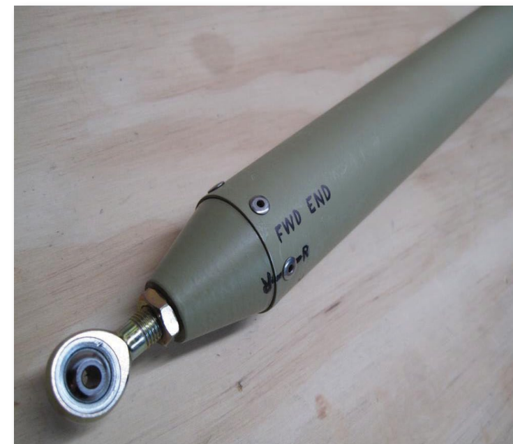
BELOW: If the lock nut is not tightened the rod end bearing will 'wobble around', allowing free play in the control system
