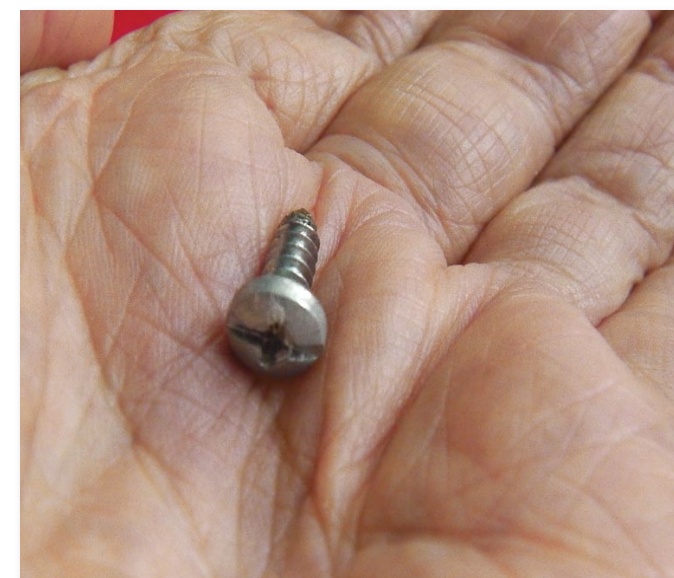
ABOVE: Sloppy airframe inspection and cleaning can allow a small item like this screw to seriously jeopardize safety.
