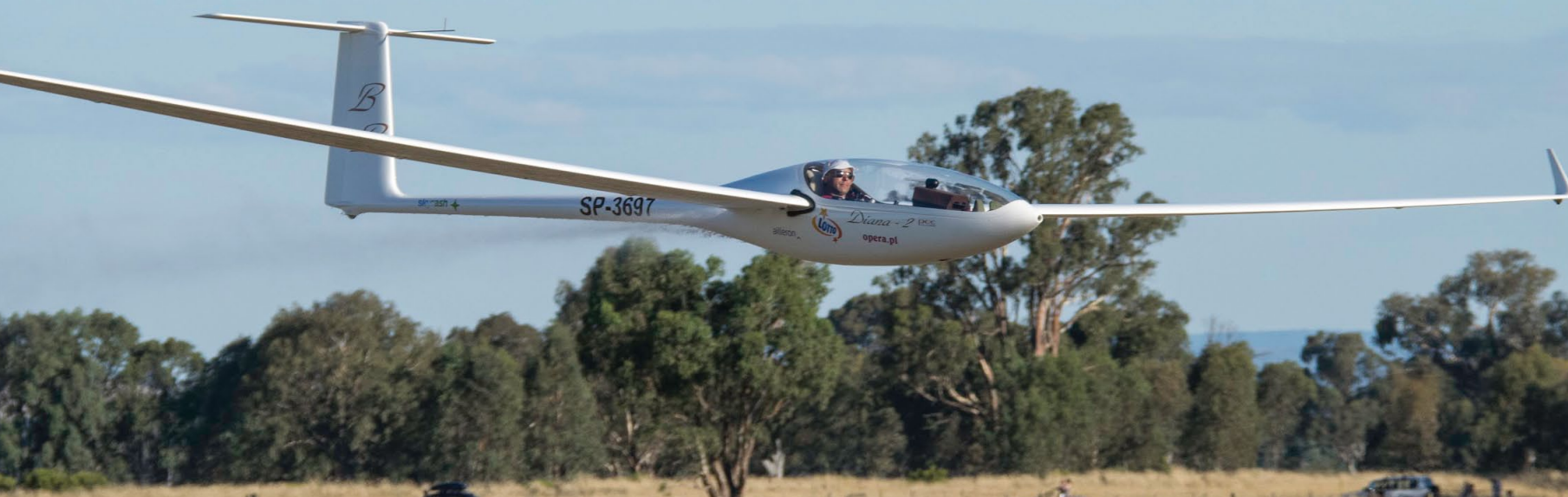
ABOVE: It is true, the wing of the Diana 2 is curved, with no straight lines at all.
