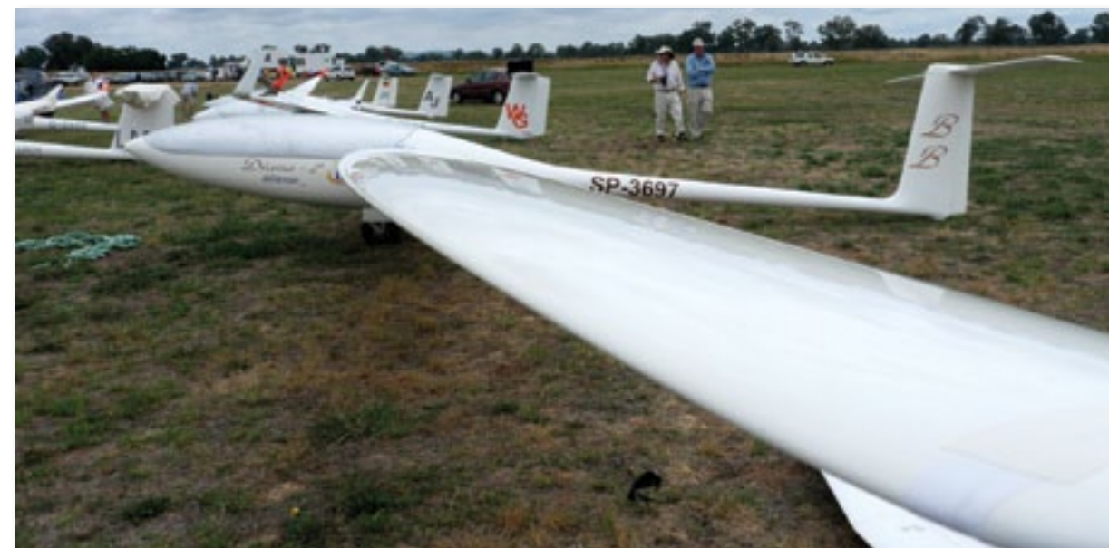
ABOVE: It is true, the wing of the Diana 2 is curved, with no straight lines at all.
